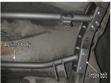
5. A series of self-tapping 3/8" bolts are used to hold the cradle in place. First drill the holes with a 5/16" bit and then thread the bolts into the frame.
